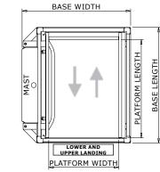
• 42 x 60 platforms meet the A18.1 requirements for maximum allowable clear platform space at 750 lbs.
